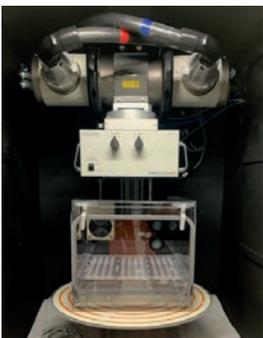
Environmental chamber to introduce and control gases. Allows variables like humidity, temperature, or hypoxic conditions, to be changed during treatment.
