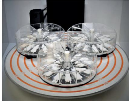
Planetary turntable holds multiple cell plates and pie cages for increased throughput. Rotation ensures uniform dose delivery.
