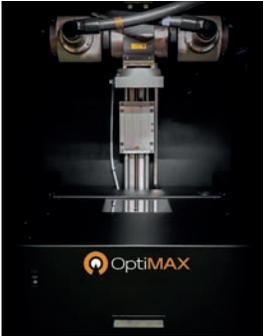
OptiMAX 2D image-guided radiotherapy module, expands capabilities by providing researchers with multi-modality imaging, including BLI, x-ray, and radioisotopic imaging.
