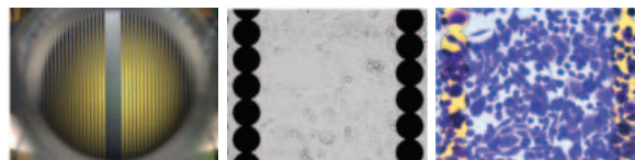
Figure 2. Left: View looking down into an E-Plate VIEW well. Center and right: Views of cells within the biosensor-free region.
