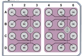
Figure 1. BioFlux 24-well plate channels.
