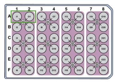
**Figure 1. 48-well BioFlux plate**. The green square highlights an inlet (A1) and outlet (A2) well with a viewing channel connecting the two wells. Each pair of inlet and outlet wells represent independent assays.
