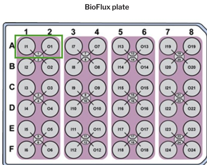
**Figure 1. 48-well BioFlux plate.** The green square highlights an inlet (A1) and outlet (A2) well with a viewing channel connecting the two wells. Each pair of inlet and outlet wells represent independent assays.
