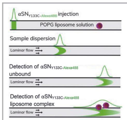
Figure 2. FIDA principle. 40 nL of the indicator,  $\alpha$ SN (labelled with alexa488 at the C-terminus), is introduced into the capillary under laminar flow. The indicator will then be dispersed proportionally to its molecular size. This principle is utilised for accurate size determination of free indicator and liposome-bound indicator.
