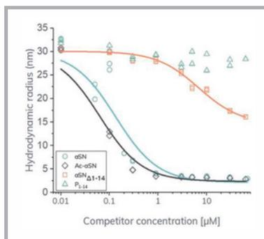
Figure 4. FIDA competition assay. The apparent size of liposome-bound  $\alpha\text{SN}$  (100  $\mu\text{M}$  POPG and 0.2  $\mu\text{M}$   $\alpha\text{SN}$ ) as a function of four different  $\alpha\text{SN}$  analogs. The data points were fitted to the FIDA binding isotherm, in order to determine  $\text{IC}_{50}$  values.
