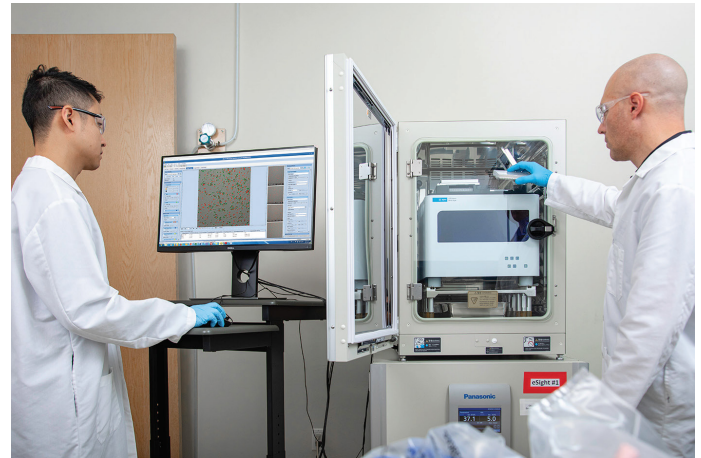
Figure 2. An Agilent xCELLigence RTCA eSight instrument is housed inside an incubator and offers a significant reduction in biohazardous exposure and plastic waste.
